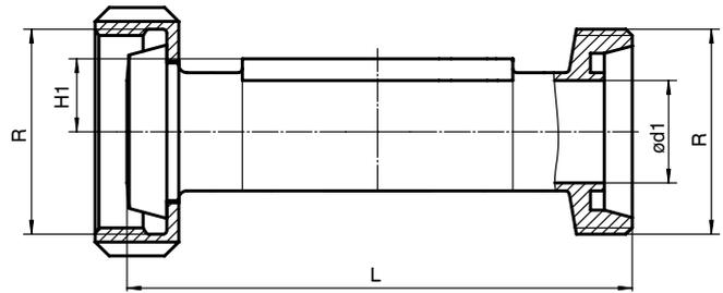
**Raccords clamps, code du raccordement 80, 82, 88, 8A, 8E**
