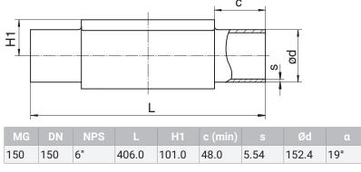
Dimensions in mm, MG = diaphragm size
