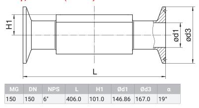
Dimensions in mm, MG = diaphragm size
